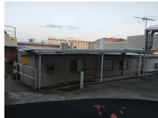
P16 ALL PAVING, BOLLARD, RETAINING WALLS & DEMOUNTABLES TO BE DEMOLISHED. SERVICES RETICULATION - REFER TO SERVICES ENGINEERS DOCUMENTATION. IF ANY ARE NEEDED TO BE RETAINED MOVE TO IN GROUND. ENGINEERS TO CONFIRM.
